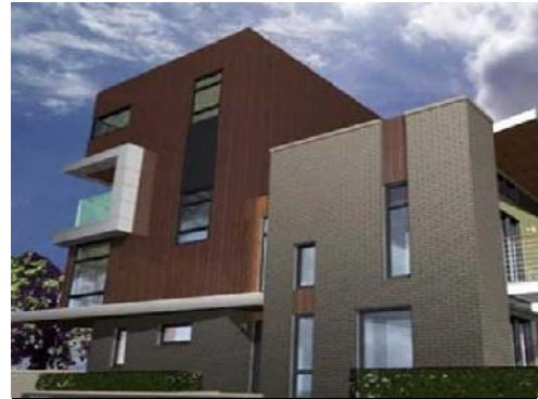
Fig. 5 Color changes & variation in material and depth are good tools to break up the massing of a building.
