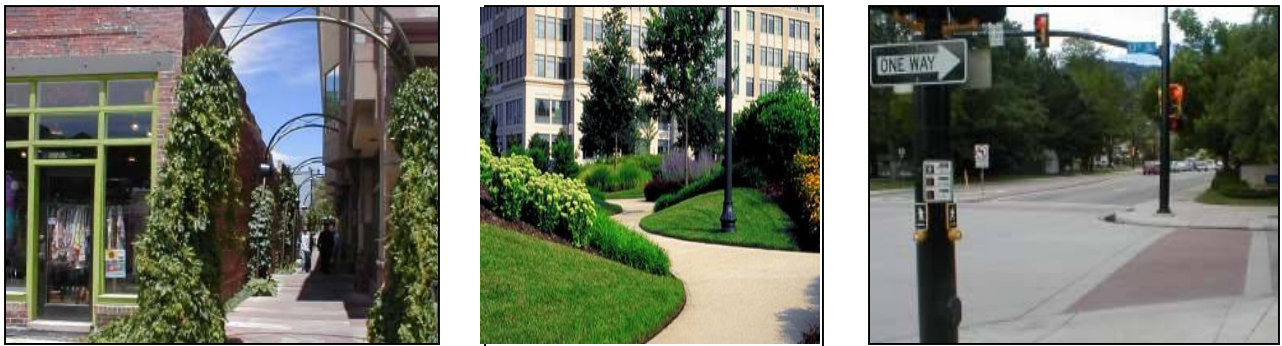
Fig. 11 Pedestrian corridors should be marked by landscaping and other treatments. Corridors provide access between buildings and parking areas. Delineating crosswalks using a different paving material or painted stripes enhances pedestrian safety and the overall streetscape.
